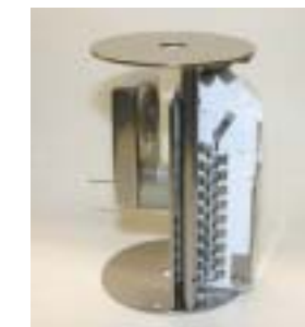
Figure 8. Photograph of a DM283 large-area HED detector.
