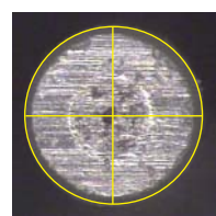
Concentricity of bores in 1/32" PEEKsil tubing. SGE PEEKsil (left) and a competitor's tubing.
