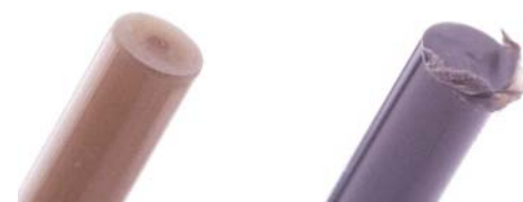
Tubing ends should be precisely square (left) to avoid volumes at the connection joint.
