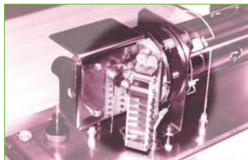
Figure 3. 14617 detector installed in an Agilent 5973 MSD
